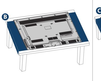
Align the screw holes on the stand column with the holes on the back of your TV, then secure the column to your TV with the four OR provided M5  $\times$  12 mm screws (the short
